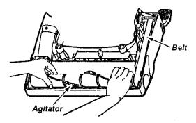
Position hands on the agitator. If the belt is still attached to the agitator, there will be tension on it.
